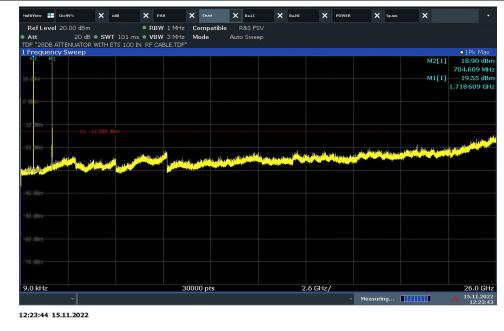
2 Bands per antenna port Conducted Spurious Emissions
