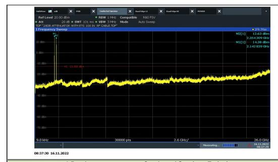
2 Bands per antenna port Conducted Spurious Emissions CU with Antenna Port A Downlink: LTE Band 25 20MHz BW Mid Ch & LTE Band 12 10MHz BW High Ch
