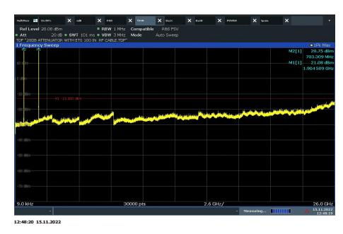
2 Bands per antenna port Conducted Spurious Emissions Antenna Port A Uplink: LTE Band 25 20MHz BW High Ch
