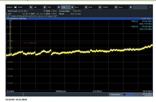
2 Bands per antenna port Conducted Spurious Emissions Antenna Port A Uplink: WCDMA Band 5 5MHz BW Mid Ch & LTE Band 30 5MHz BW High Ch
