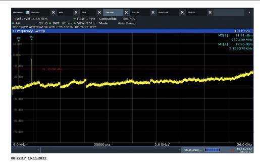
2 Bands per antenna port Conducted Spurious Emissions CU with Antenna Port A Downlink: LTE Band 4 20MHz BW High Ch & LTE Band 30 10MHz BW Mid Ch
