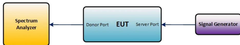
Figure 3 – Downlink test configuration in EUT test mode
