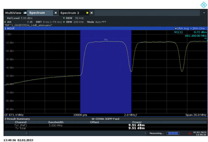
WCDMA Band 5 15MHz bandwidth DL Low channel Output power / channel
