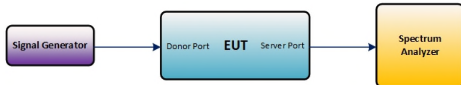
Figure 3 – Downlink test configuration in EUT test mode
