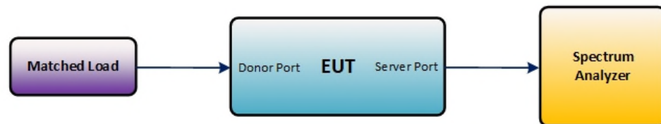
Figure 6 – Maximum downlink noise limit test configuration
