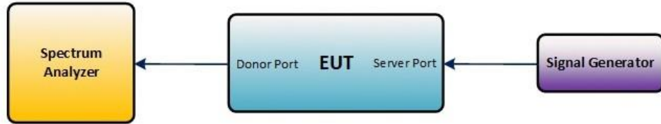
Figure 3 – Downlink test configuration in EUT test mode
