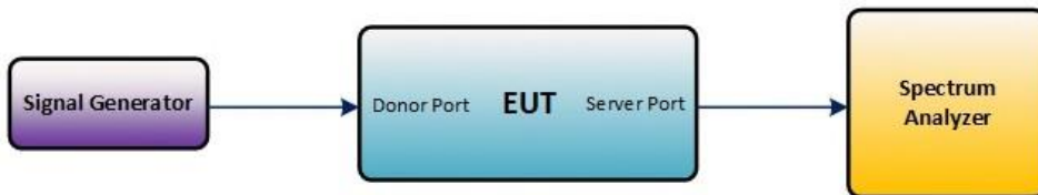
Figure 5 – Intermodulation product instrumentation test setup
