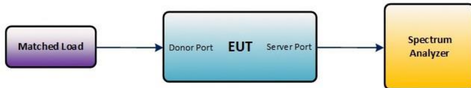
Figure 6 – Maximum downlink noise limit test configuration
