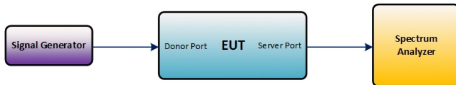
Figure 5 – Intermodulation product instrumentation test setup
