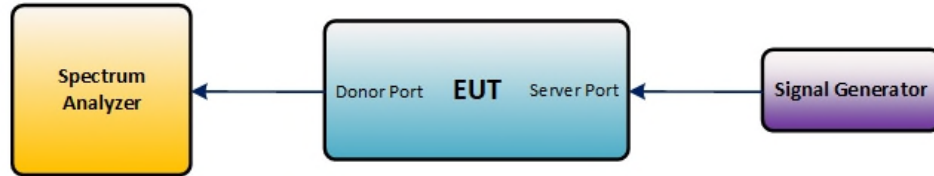
Figure 3 – Downlink test configuration in EUT test mode
