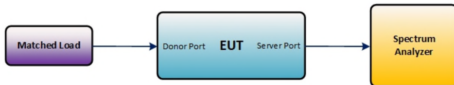
Figure 6 – Maximum downlink noise limit test configuration
