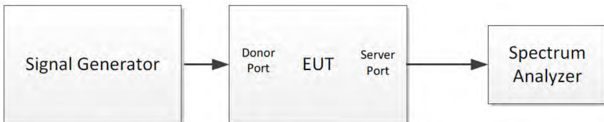
Figure 3 – Downlink test configuration in EUT test mode
