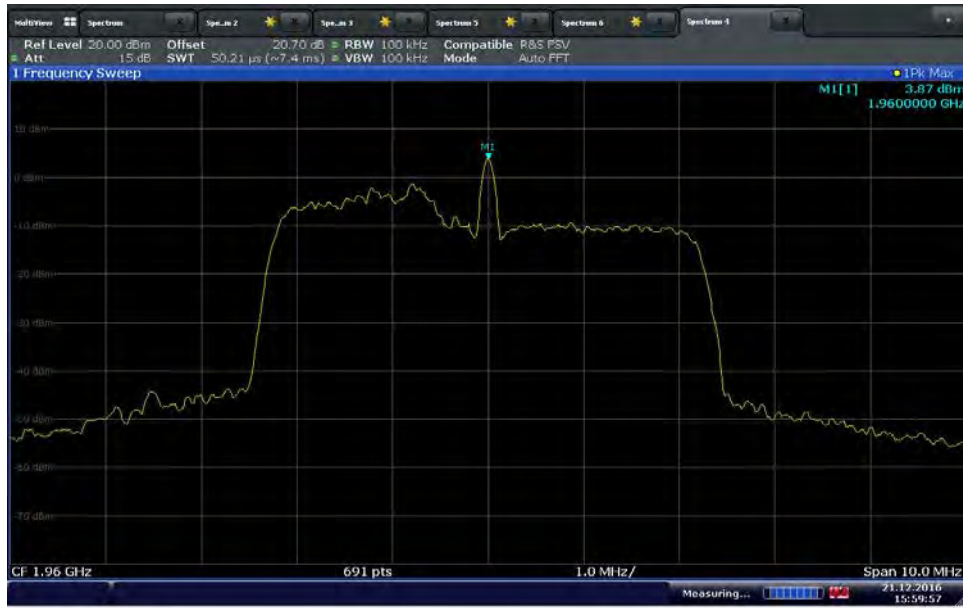
WCDMA B2 Downlink Mid Channel 120VAC @ 20°C
