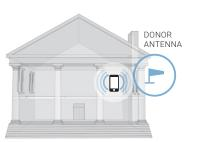
Install **Donor Antenna** where the mobile device receives this signal.
