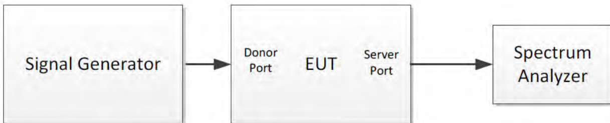
Figure 3 – Downlink test configuration in EUT test mode
