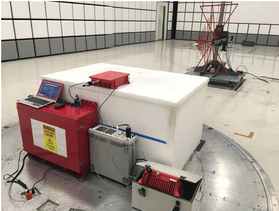
CU Radiated Emissions Below 1GHz Rear
