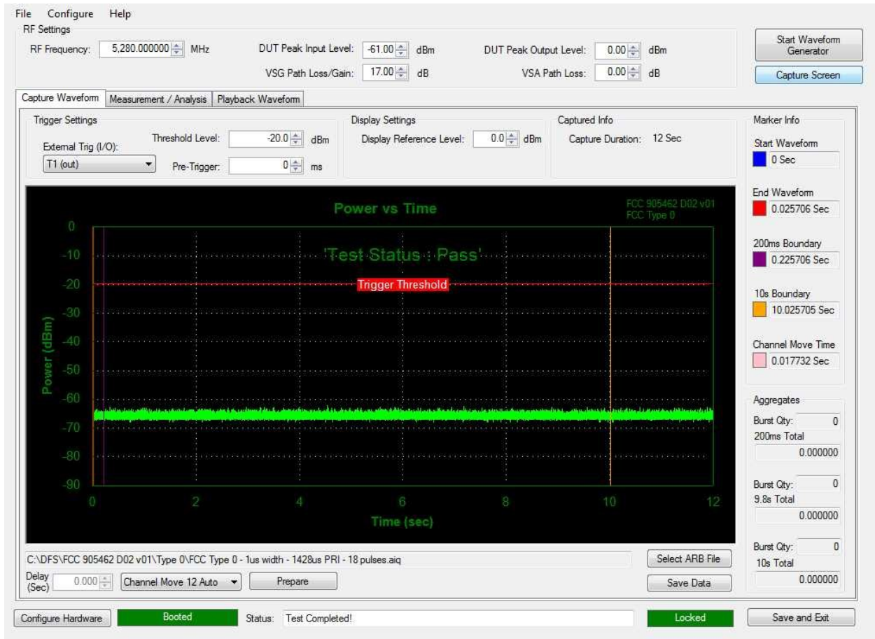
5280 MHz Overall Power vs Time Display, showing 10 seconds observation time
