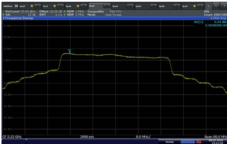
UNII 1 40MHz Bandwidth Mid Channel 5220 MHz
