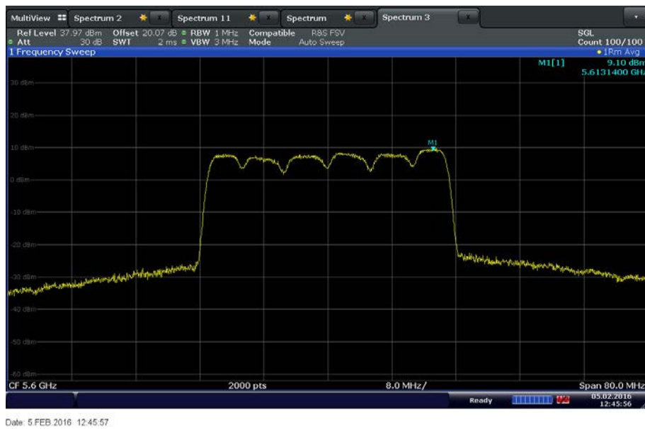
UNII 2C 30MHz Bandwidth Middle Channel 5600 MHz
