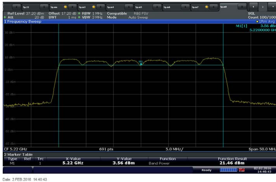
UNII 1 30MHz Bandwidth Middle Channel 5220 MHz
