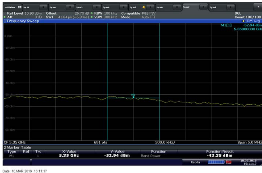
UNII 2A 30MHz Upper Band Edge 5350MHz (Average Measurement) @ 5310 MHz
