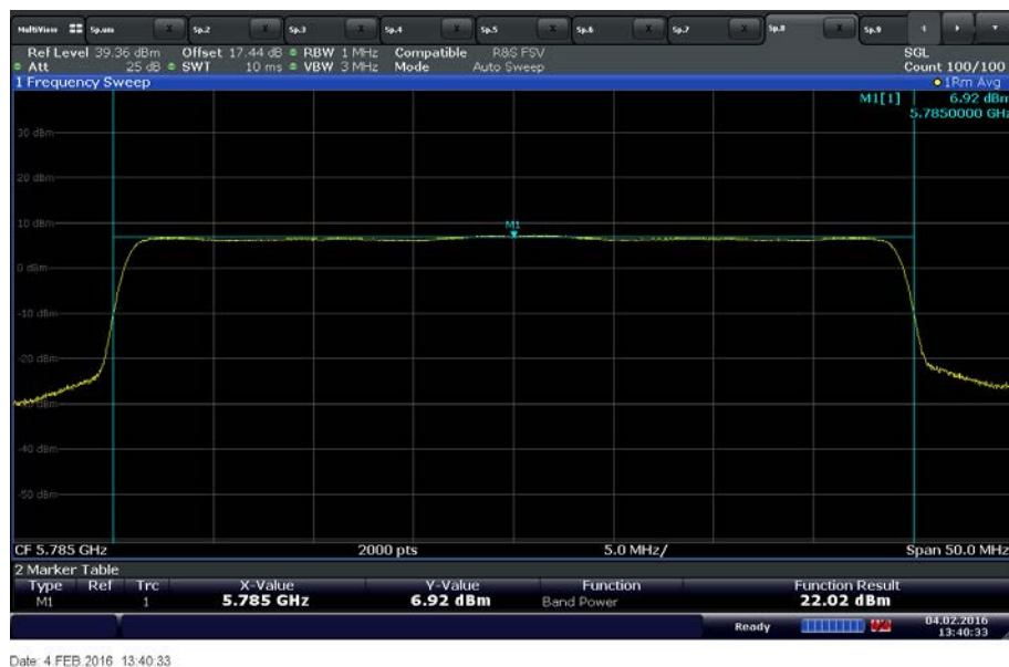
UNII 3 40MHz Bandwidth Middle Channel 5785 MHz
