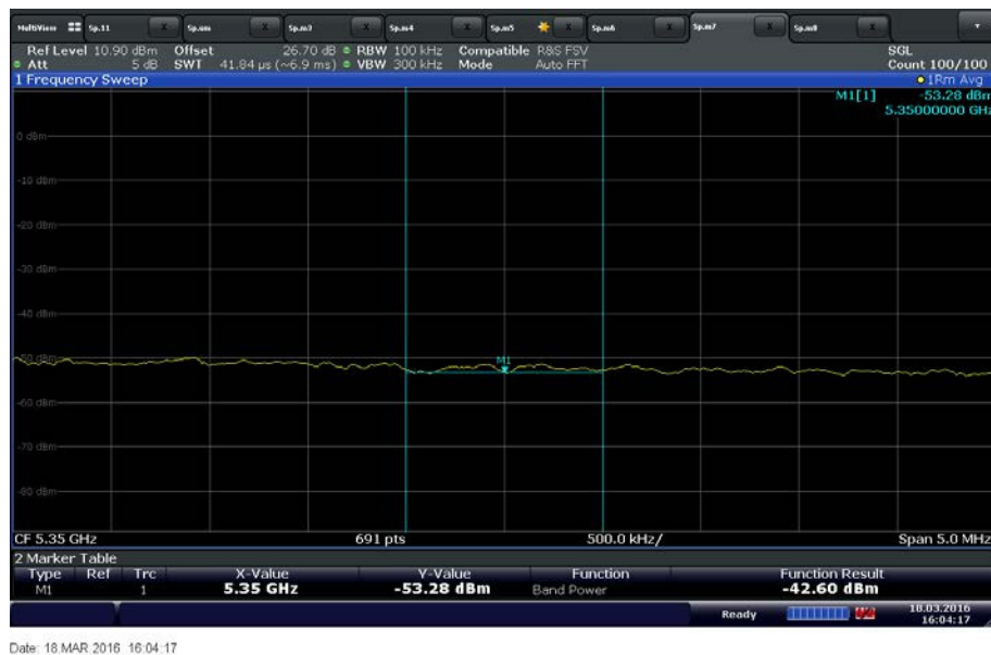
UNII 2A 40MHz Upper Band Edge 5350MHz (Average Measurement) @ 5310 MHz
