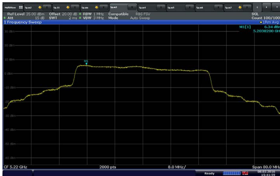
UNII 1 40MHz Bandwidth Mid Channel 5220 MHz
