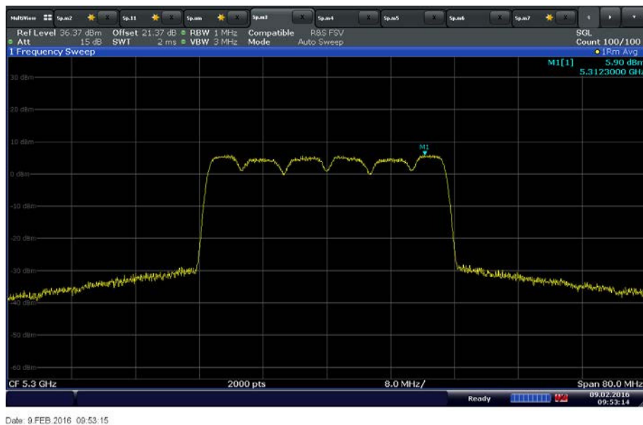
UNII 2A 30MHz Bandwidth Middle Channel 5300 MHz
