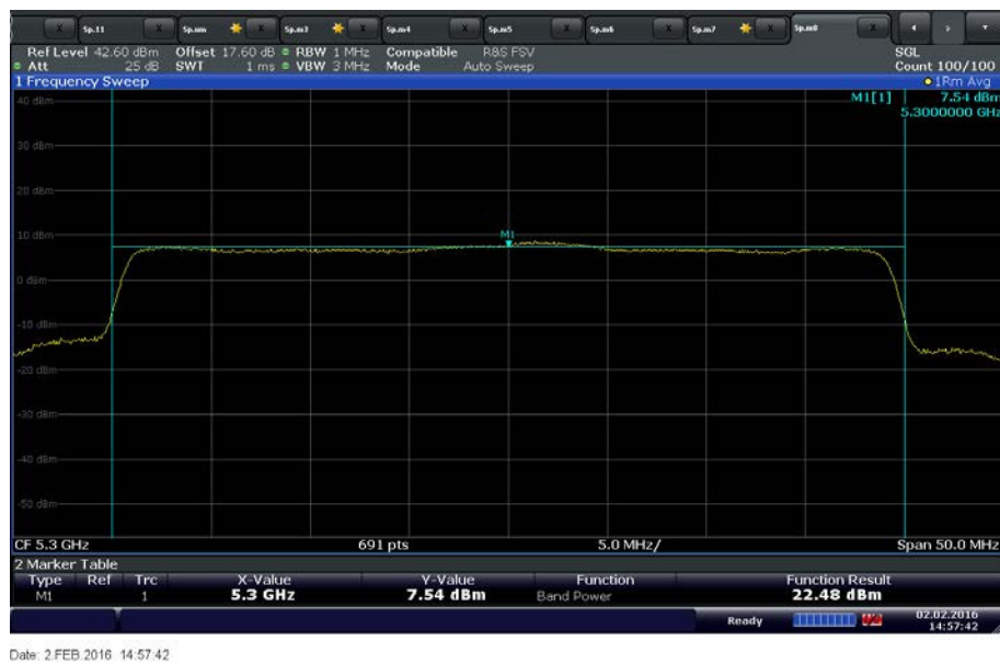
UNII 2A 40MHz Bandwidth Middle Channel 5300 MHz
