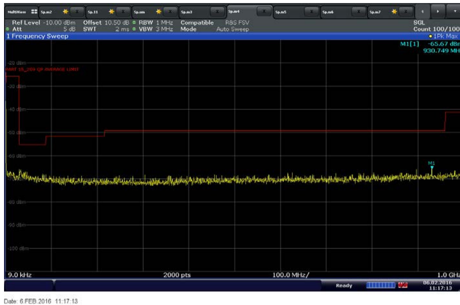
UNII 1 30MHz Bandwidth Middle Channel 5220 MHz Below 1GHz
