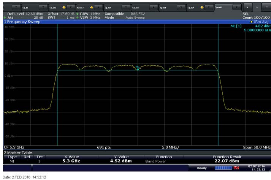
UNII 2A 30MHz Bandwidth Middle Channel 5300 MHz
