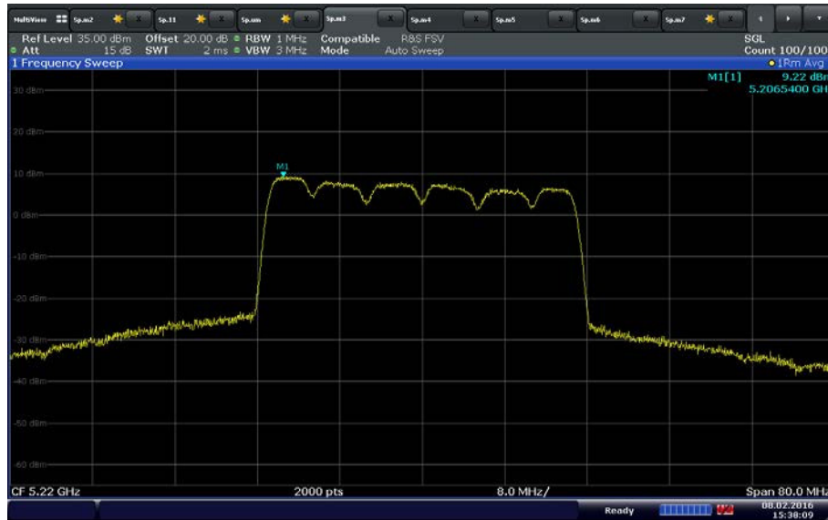
UNII 1 30MHz Bandwidth Middle Channel 5220 MHz
