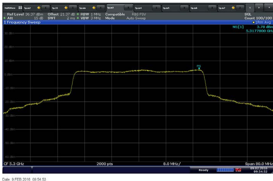
UNII 2A 40MHz Bandwidth Middle Channel 5300 MHz
