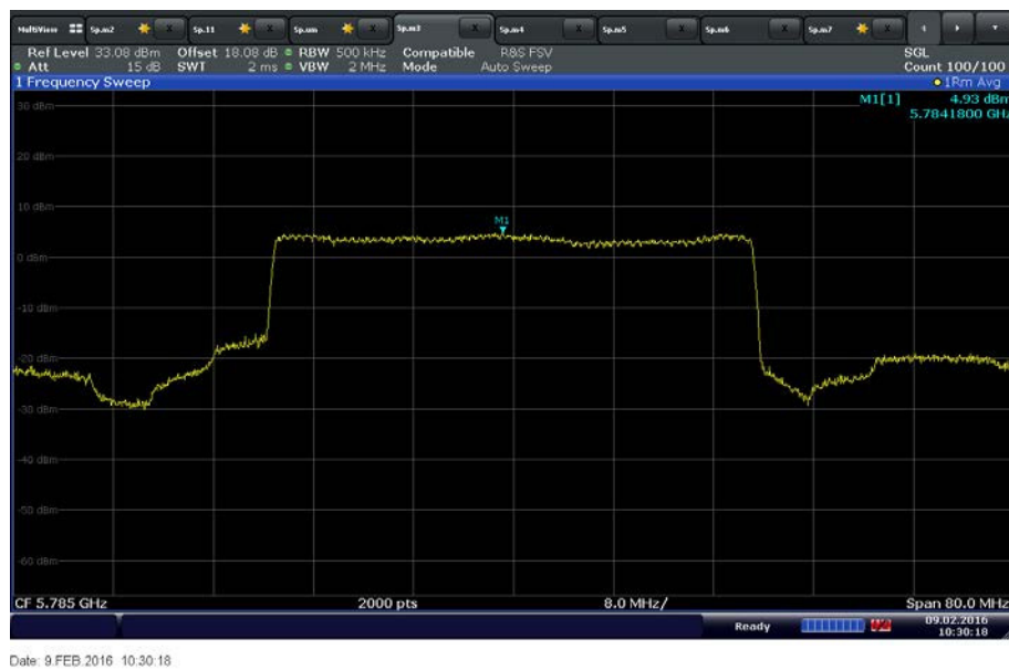
UNII 3 40MHz Bandwidth Middle Channel 5785 MHz
