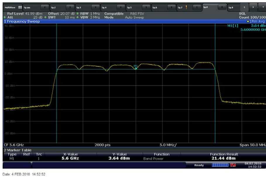
UNII 2C 30MHz Bandwidth Middle Channel 5600 MHz
