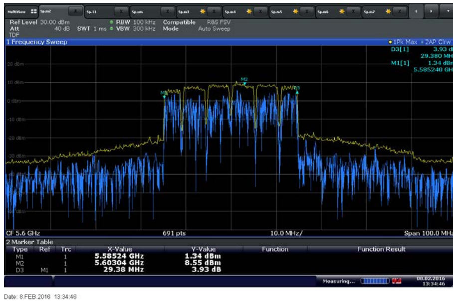
UNII 2C 30MHz Bandwidth Middle Channel 5600 MHz
