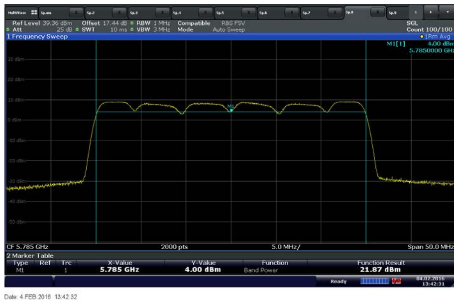
UNII 3 30MHz Bandwidth Middle Channel 5785 MHz
