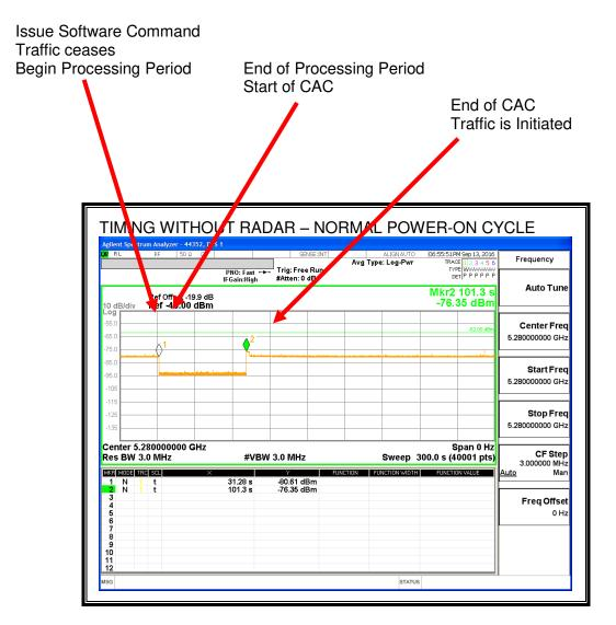
Transmissions begin on channel after completion of the initial power-up cycle and the CAC.
