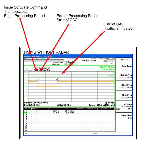
Transmissions begin on channel after completion of the initial processing period and CAC.
