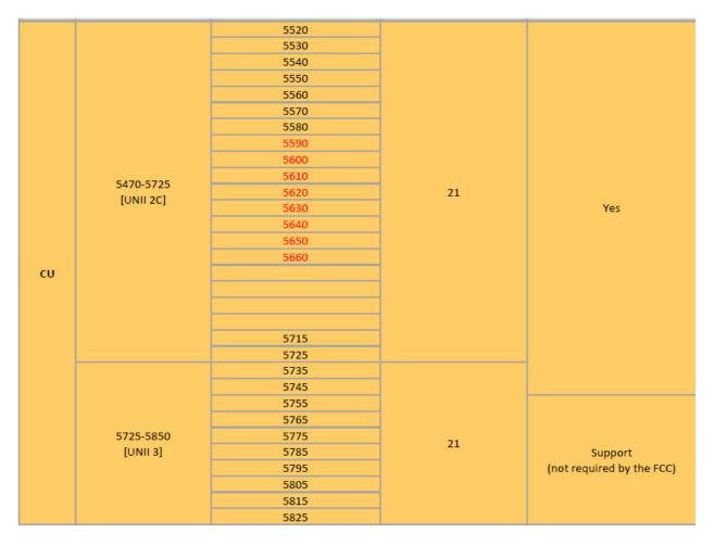
**Note:** Frequencies that overlap or reside within the 5600-5650 MHz TDWR weather band are not supported and shown in red.
