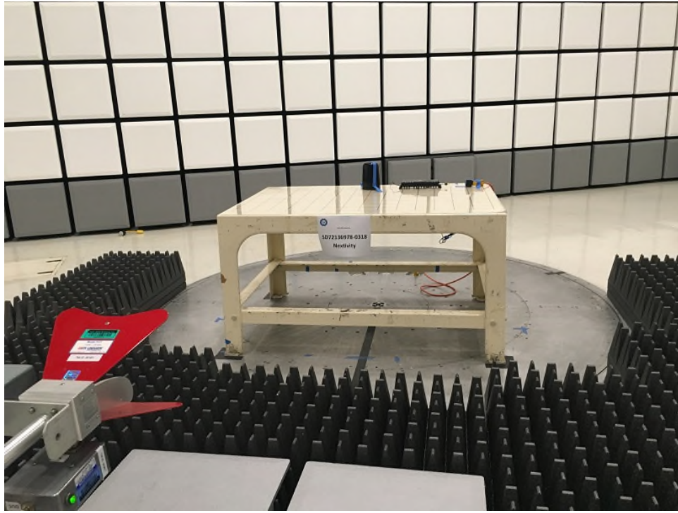
Radiated Emissions Above 1GHz Front (Standby Mode)
