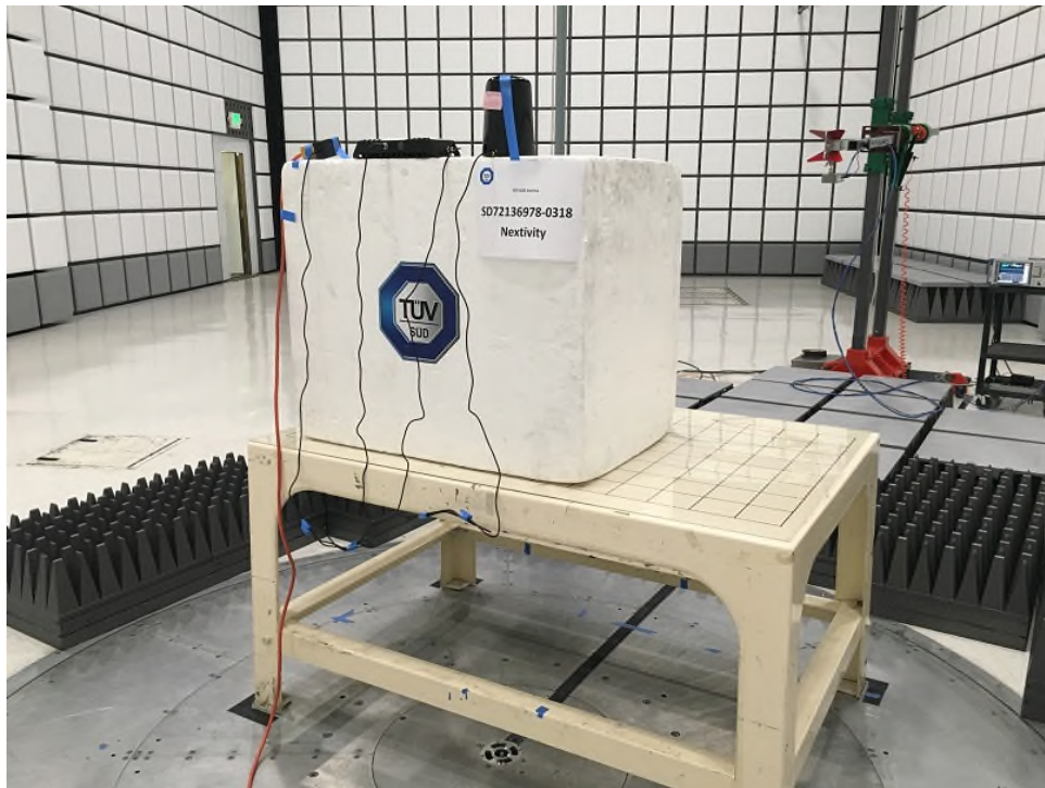
Radiated Emissions Above 1GHz Rear (Transmit Mode)
