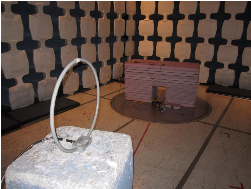
9kHz-1MHz, Y-orientation of antenna
