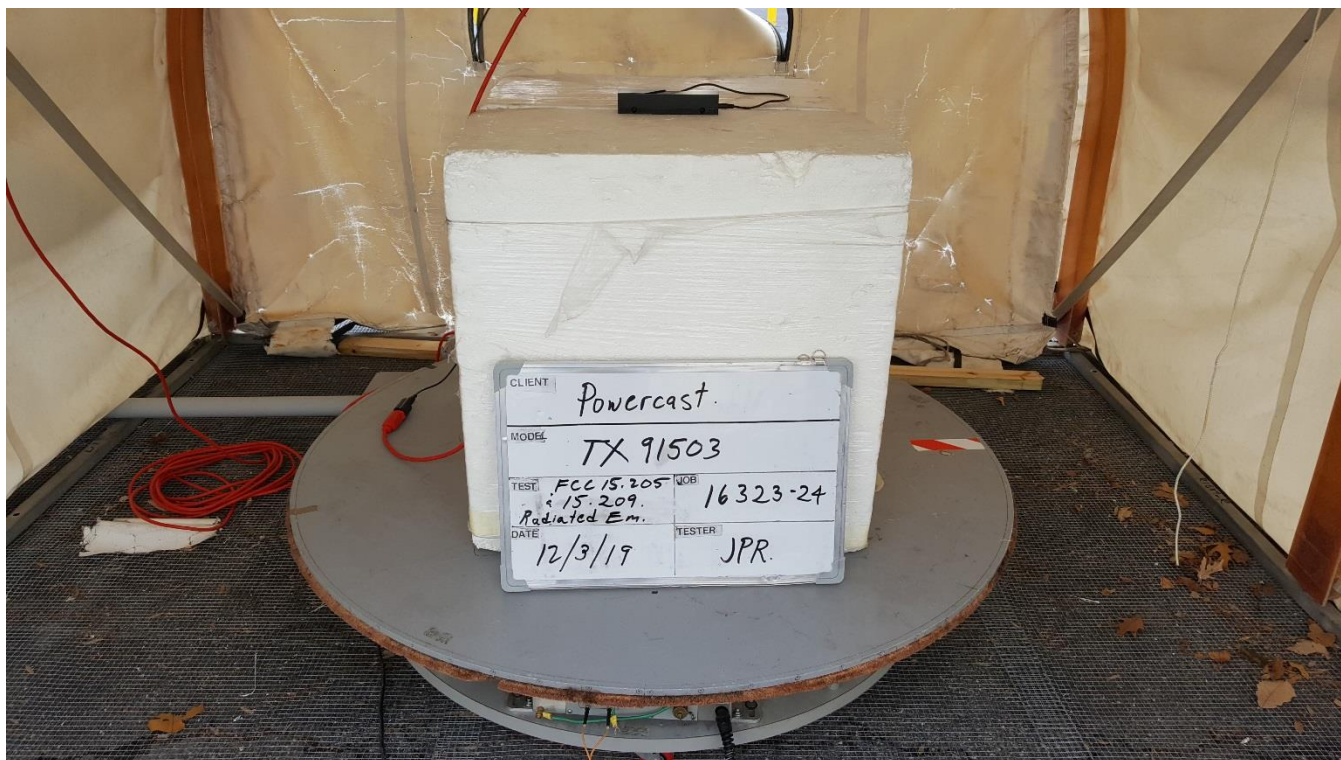
Photograph 2: Radiated Emissions Test Configuration – Flat
