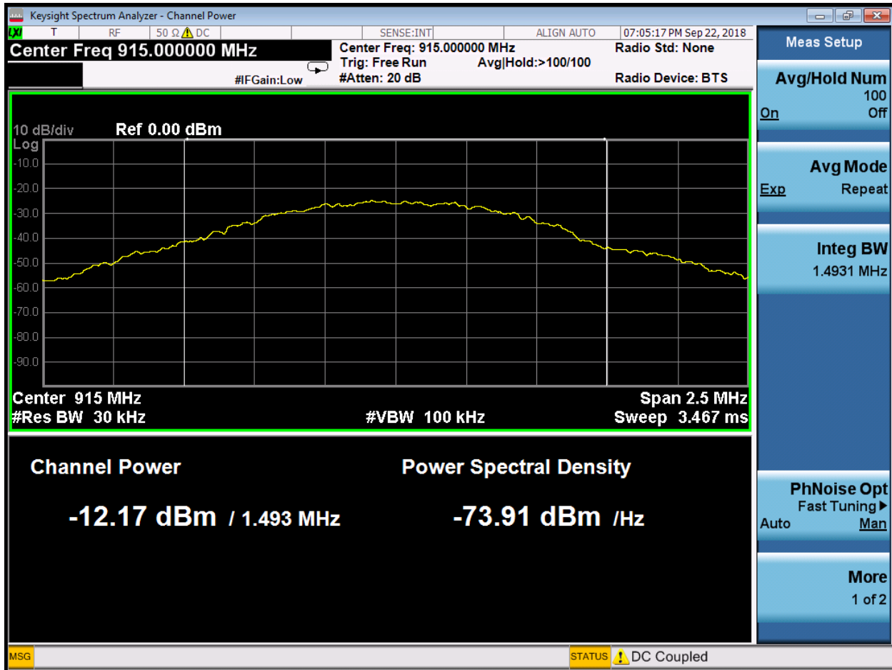
Low Data Rate Fundamental Emission Output Power
