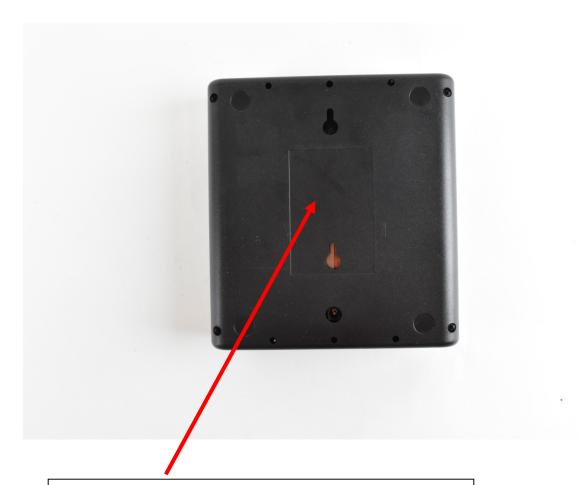
The label is placed on the back of the device in the recessed area as shown in the picture above.
