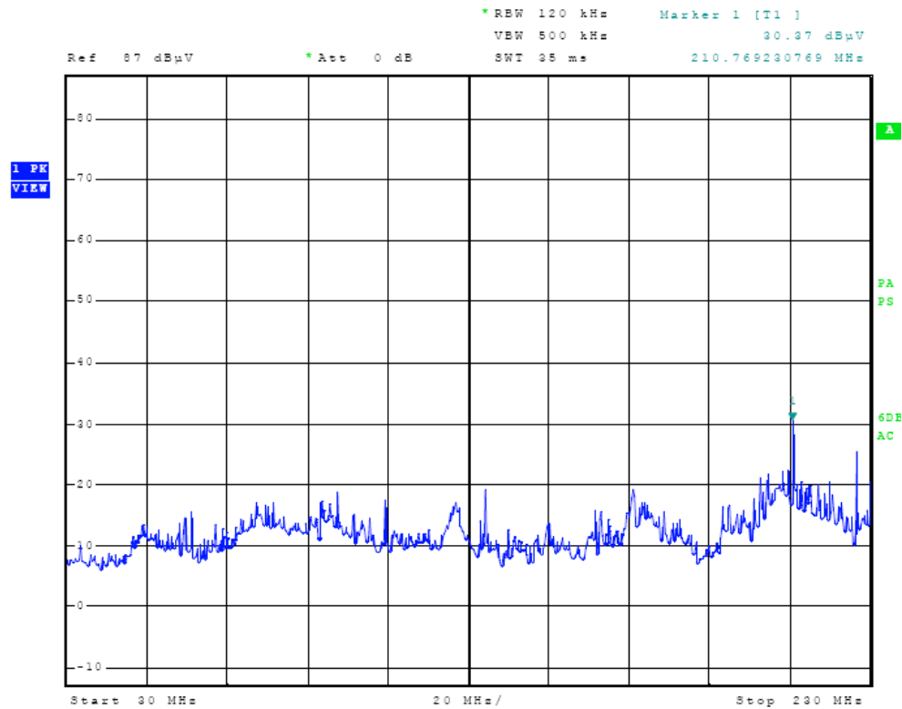
Figure One General Radiated Emissions in screen room
