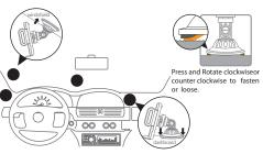
The smart pad design on the bottom of suck allows you to fix cradle on dashboard tightly
