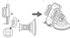
2. Press the suction and clockwise rotate the ring to Install CF-3501FMXP on a windshield or dashboard.
