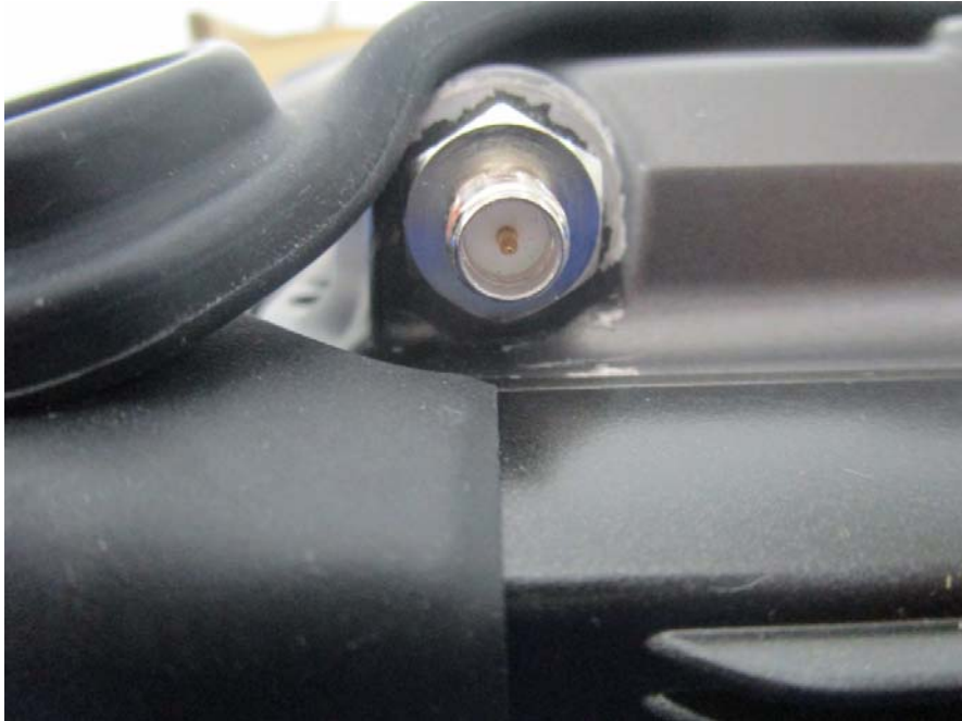
EUT – Long Range BT Antenna Port View
