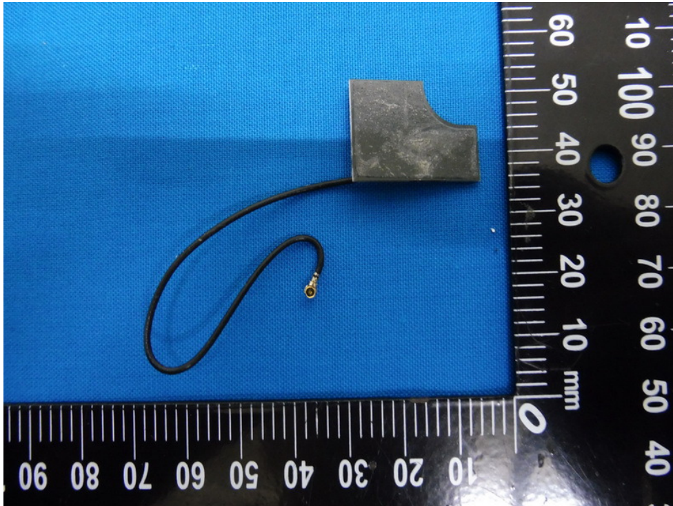
EUT BT& WiFi AUX Antenna location View
