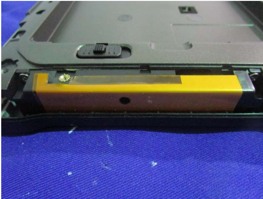
EUT -LTE&CDMA Antenna 2 View
