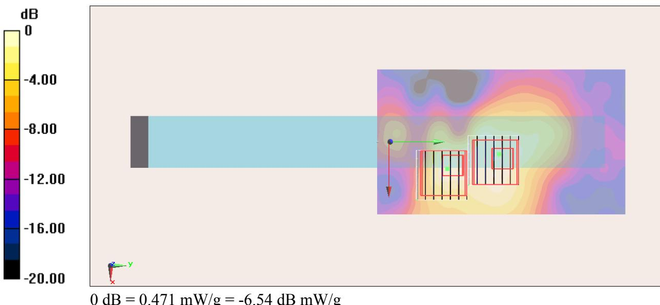
**#41\_WLAN5G\_802.11n-HT20\_Bottom Face\_0cm\_Ch149;Ant 0+1****DUT: 322149-01**
