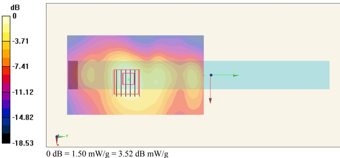
**#08\_WLAN5G\_802.11n-HT20\_Bottom Face\_0cm\_Ch36;Ant 0+1****DUT: 322149-01**
