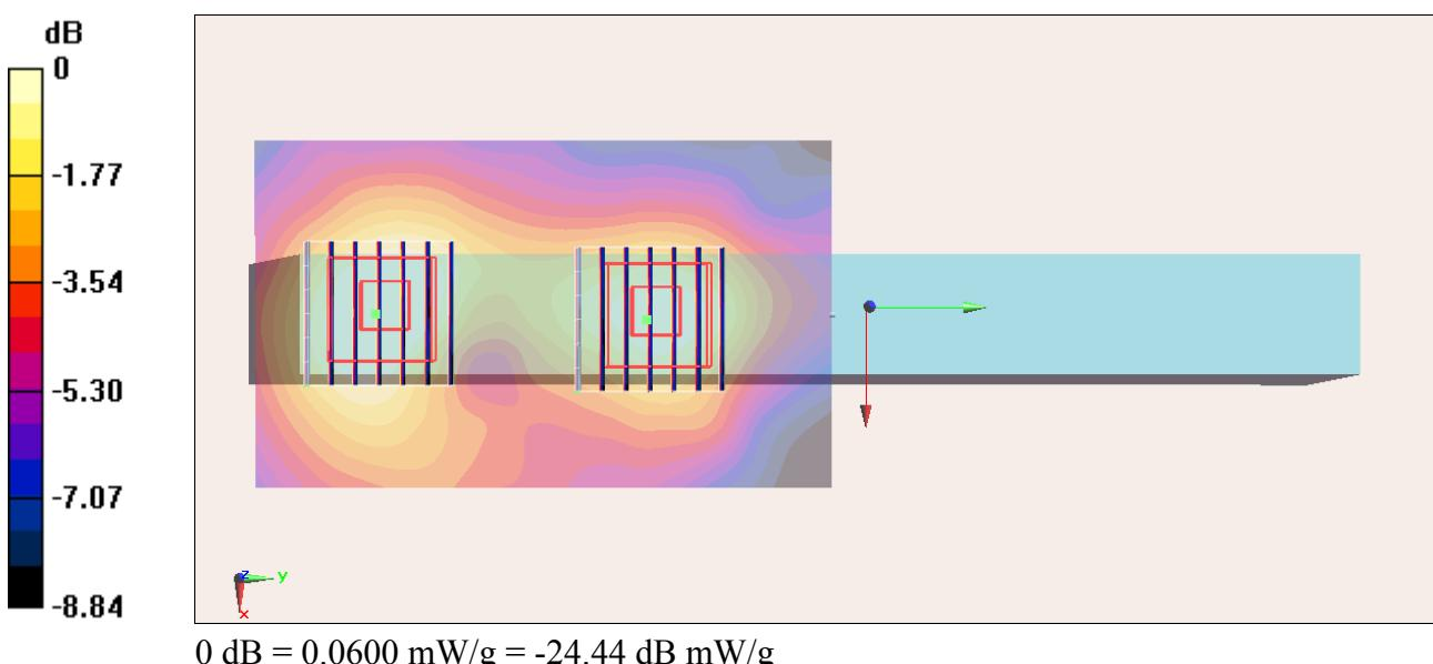
**#52\_WLAN2.4G\_802.11n-HT20\_Bottom Face\_0cm\_Ch6;Ant 0+1****DUT: 322149-01**
