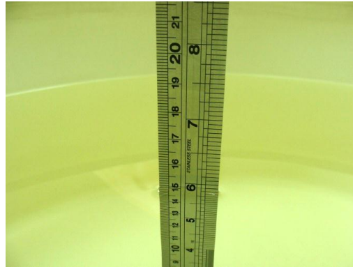
Fig 6.1 Photo of Liquid Height for Body SAR
