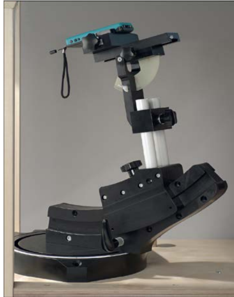
F-2. Device Holder for Transmitters
