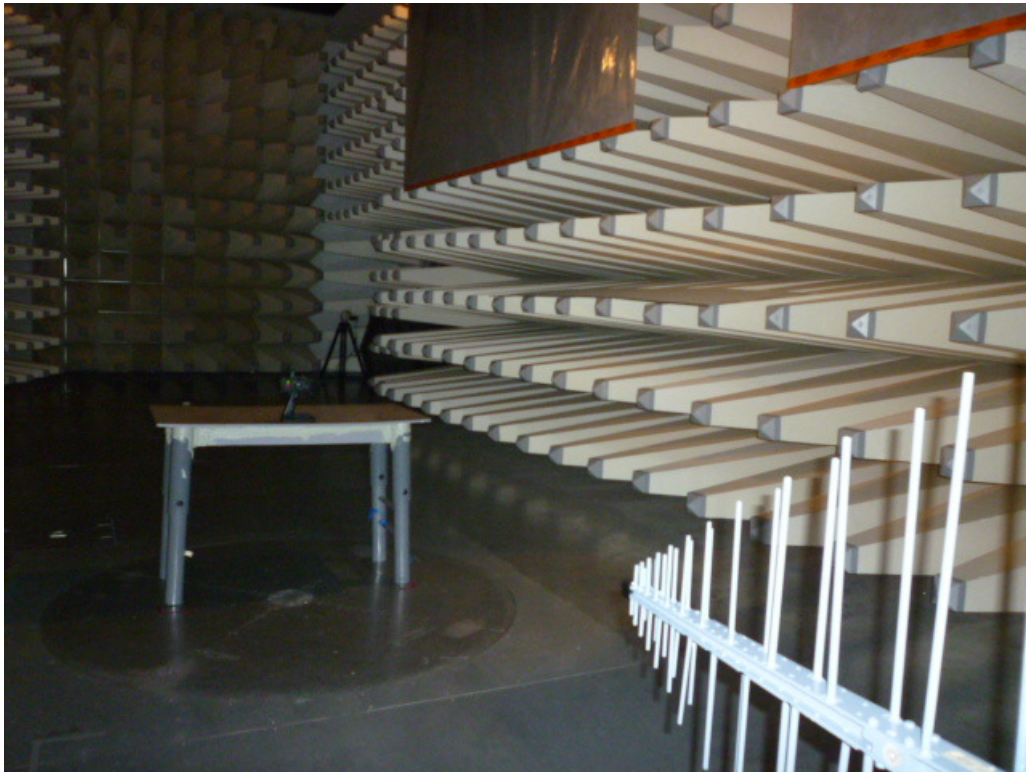
Set-up for Radiated Emission
