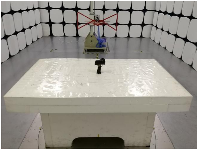
Radiated Spurious Emissions Test Setup Below 1GHz
