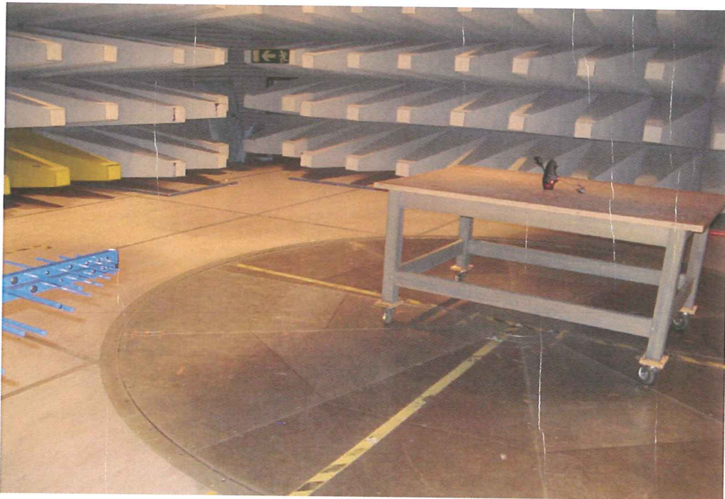
Photo 4.8.1 Test setup regarding measurement of spurious emission.
