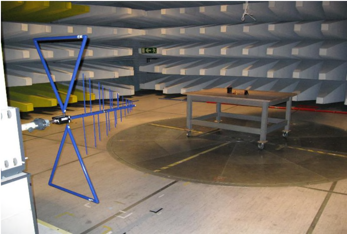
Photo 4.7.1 Test setup regarding measurement of radio frequency electromagnetic field in the measurement in the frequency span 30-1000 MHz.
