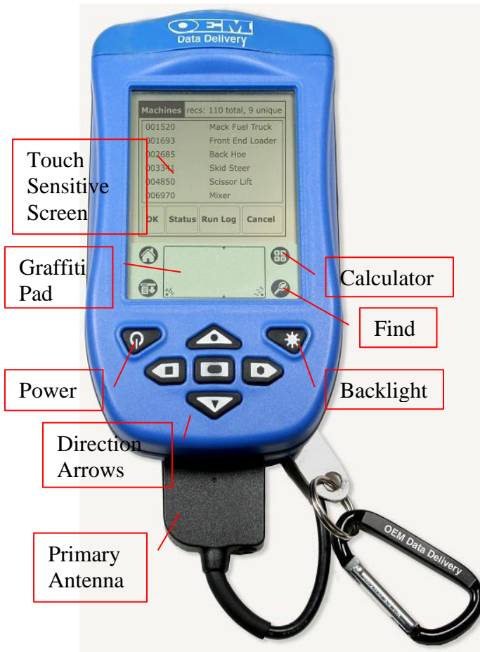
Figure 12.- Setting the ST-550 Radio Tracker Program
