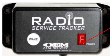
Figure 11.- ST-550 Fast and Slow Pulse Display
