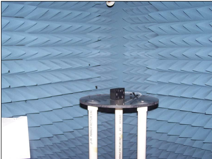
Photograph 5. Radiated Spurious Emissions, Test Setup, Above 1 GHz
