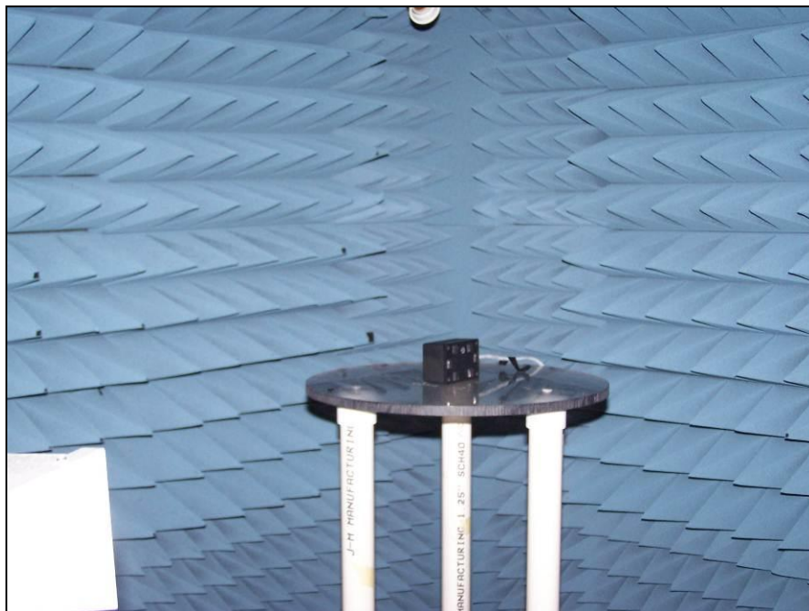
Photograph 6. Radiated Spurious Emissions, Test Setup, Above 1 GHz
