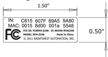
The label is placed on the back of our device:
