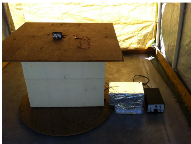
Bottom Left: AC Mains Conducted emissions test set-up
