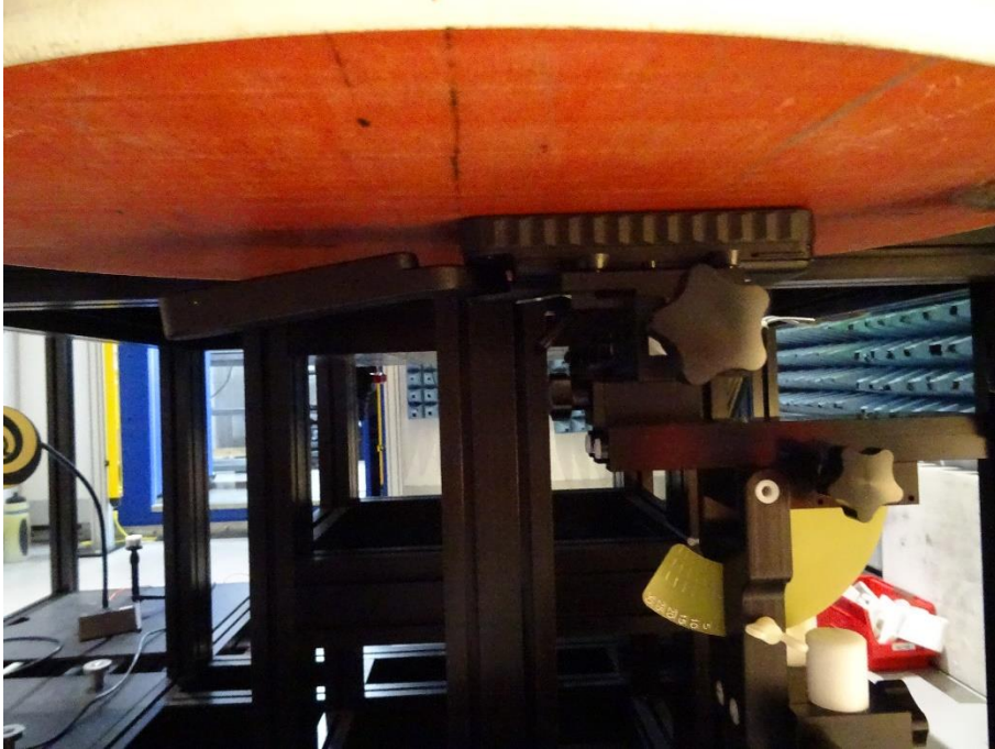
Figure 7: EUT against Elliptical Flat Phantom – 0mm separation distance
