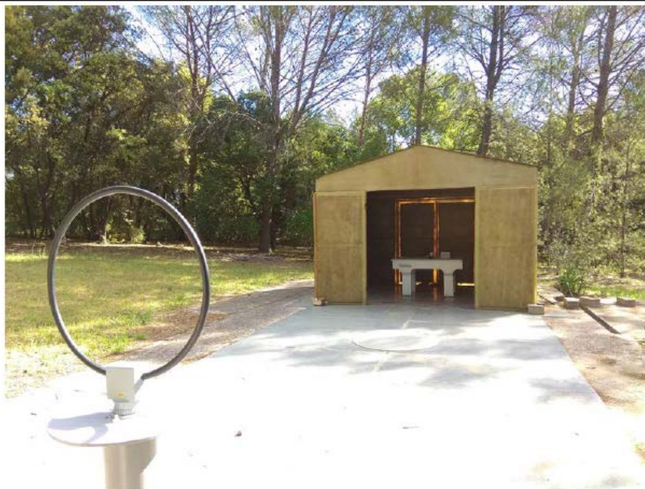
TEST SETUP PHOTO(S) RADIATED EMISSION(F<30MHZ, FINAL MEASUREMENT)
