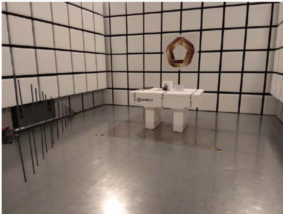
TEST SETUP PHOTO(S) RADIATED EMISSIONS (200MHZ-1GHZ)
