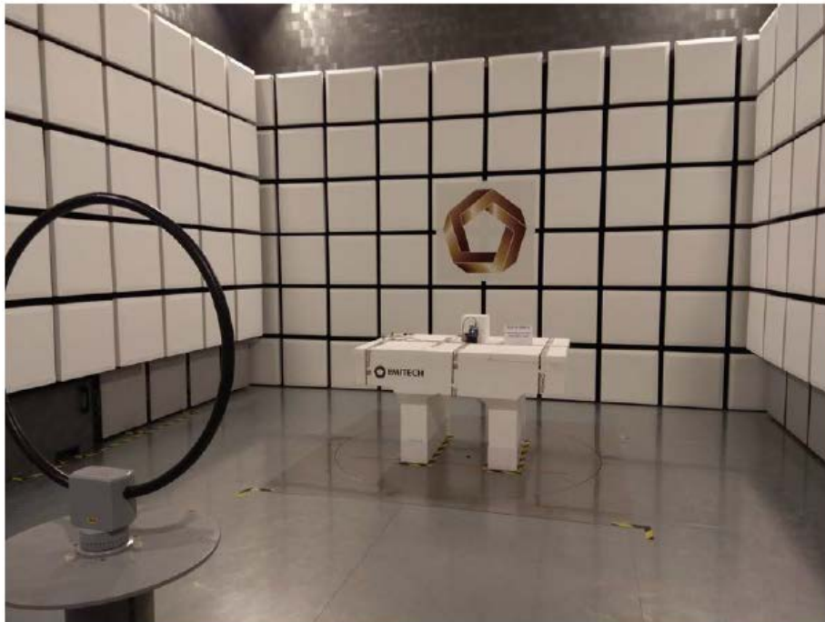
TEST SETUP PHOTO(S) RADIATED EMISSION(F<30MHZ, PRE MEASUREMENT)
