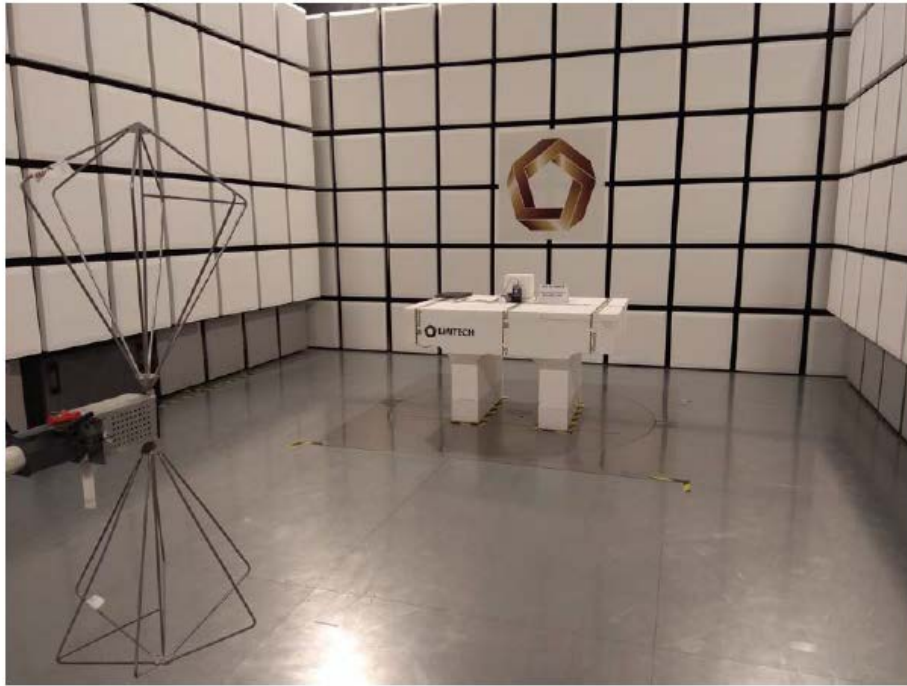
TEST SETUP PHOTO(S) RADIATED EMISSIONS (30MHZ-200MHZ)
