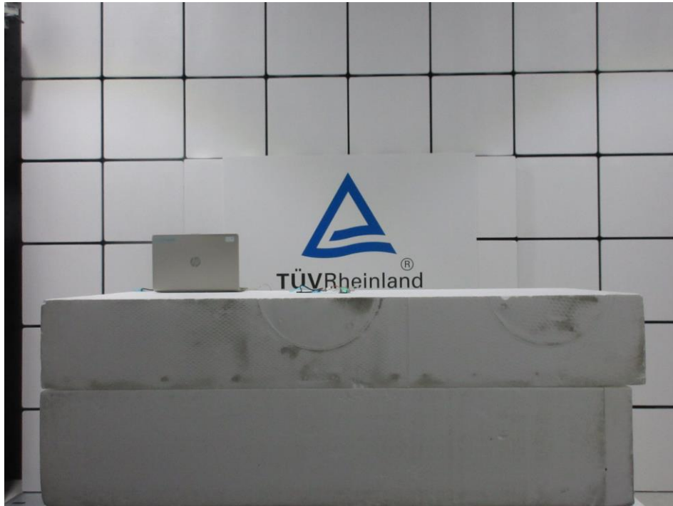
Photograph 1: Set-up for Spurious Emissions (Front View 1)
