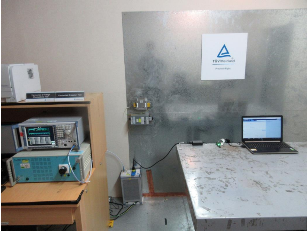
Photograph 7: Set-up for AC Mains Conducted testing (Front View)
