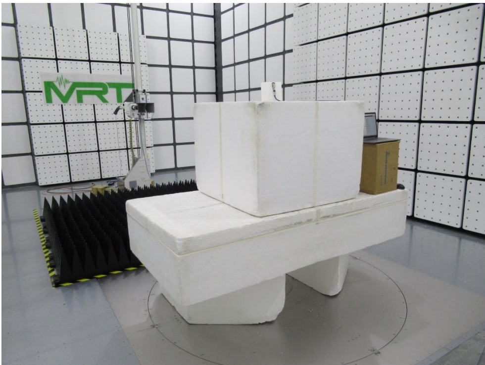
Description: Radiated Emission Test Setup for 1GHz~18GHz
