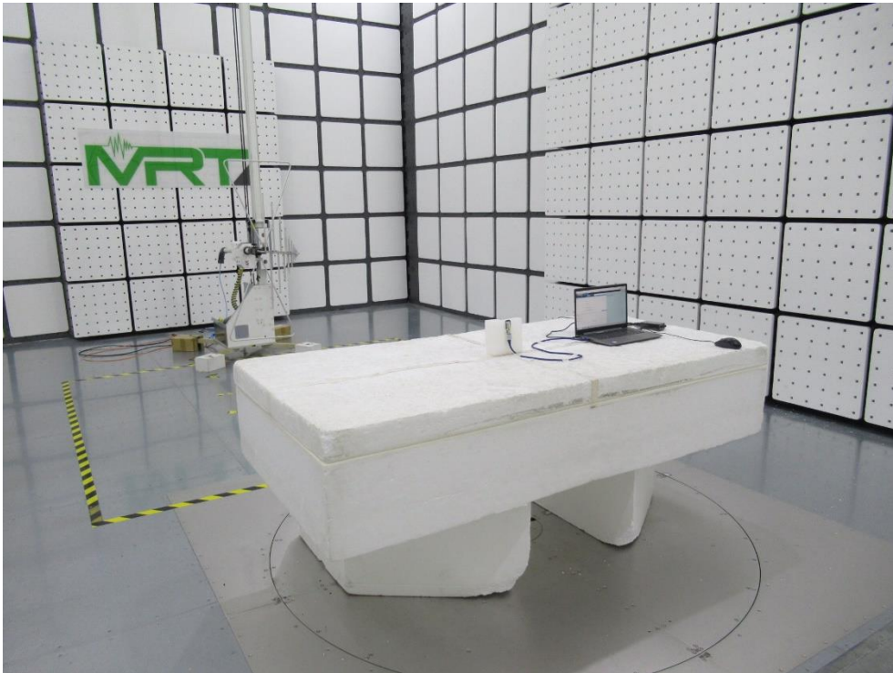
Description: Radiated Emission Test Setup for 1GHz~18GHz
