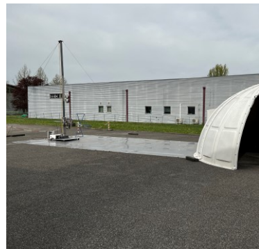
OATS Test setup (Biconic and Bi-Log antenna)
