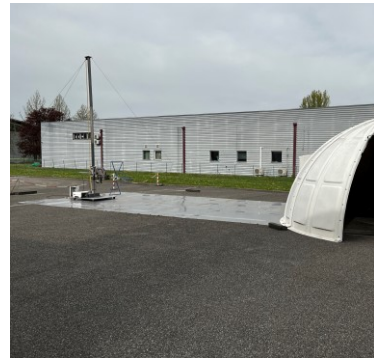
OATS Test setup (Biconic and Bi-Log antenna)
