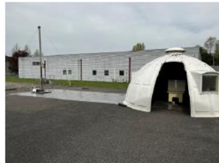
OATS Test setup (Biconic and Bi-Log antenna)
