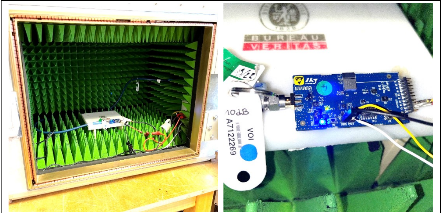
Photograph for Unwanted Emission into non-restricted frequency bands at the band edge
