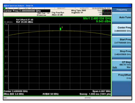
Test Plots (8DPSK) Peak Power (CH.0)
