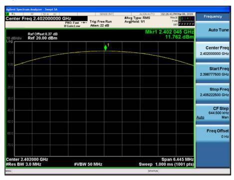
Test Plots (π/4DQPSK) Peak Power (CH.39)
