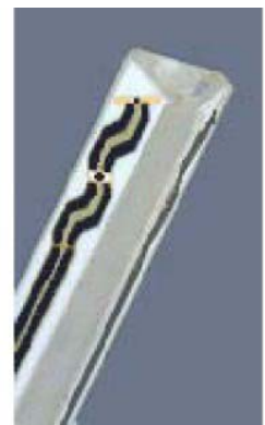
Figure 3.3 Probe Thick-Film Technique
