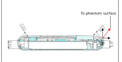
Test position B: Laptop Model : PSME4K-014001 (Front Curve)
