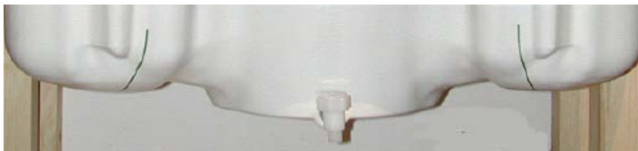
Figure 7.2 SAM Twin Phantom shell
