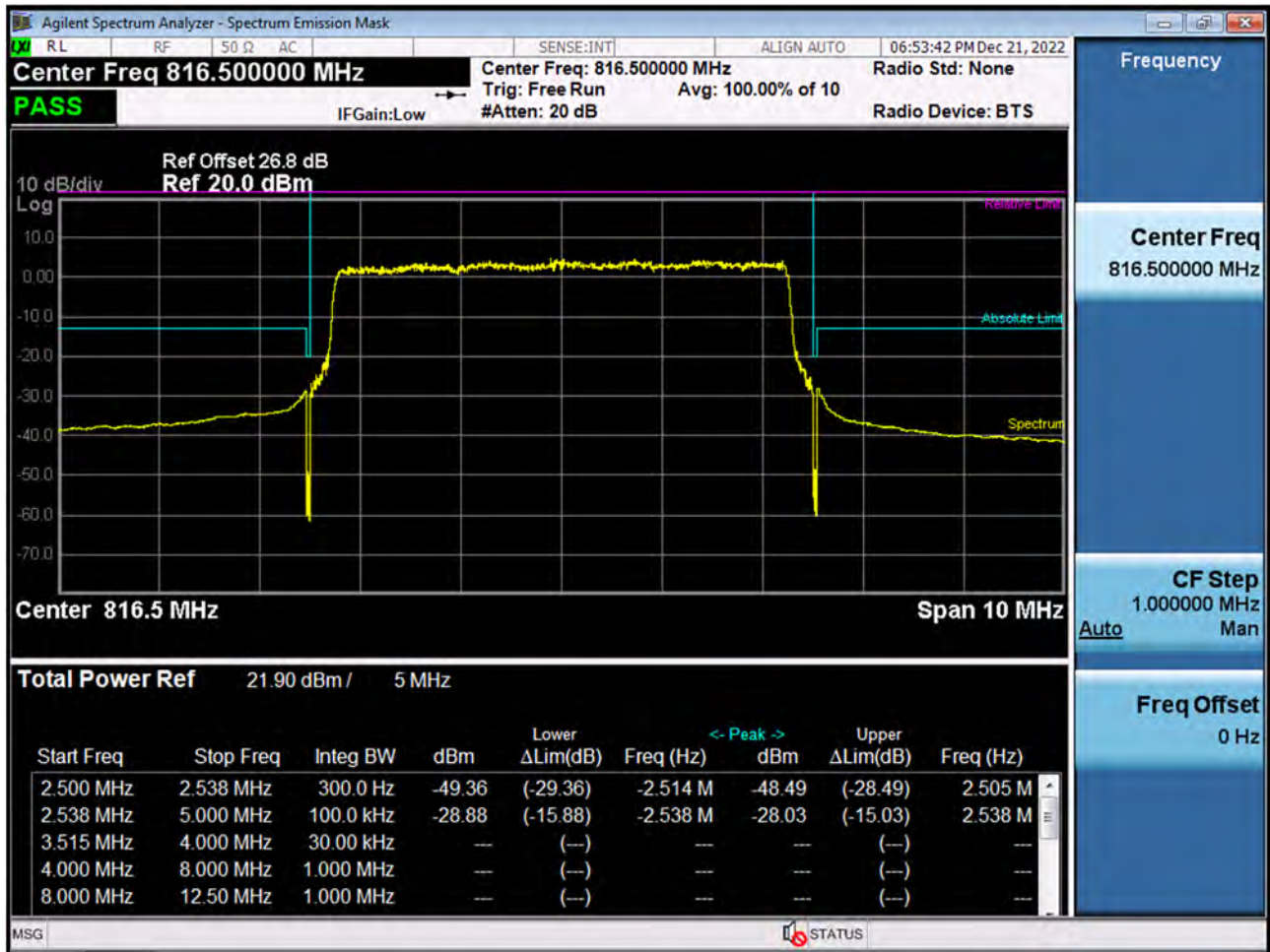
BAND 26. Upper Channel Edge Plot (5 M BW Ch.26765 QPSK_RB25_Offset 0)
