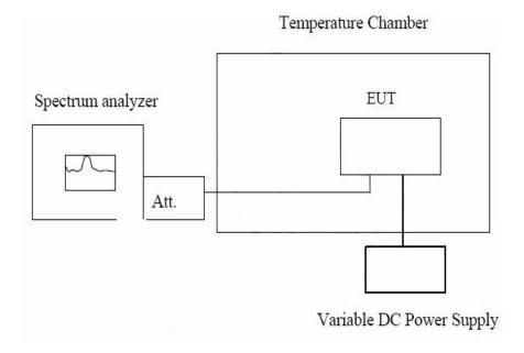
Note: Measurement setup for testing On antenna connector.
