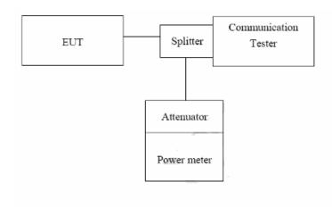
Measurement Setup for testing on Antenna connector.
