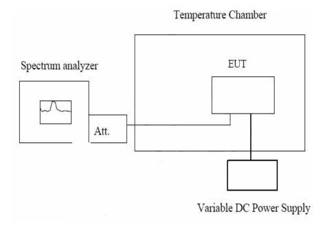
Note: Measurement setup for testing On antenna connector.
