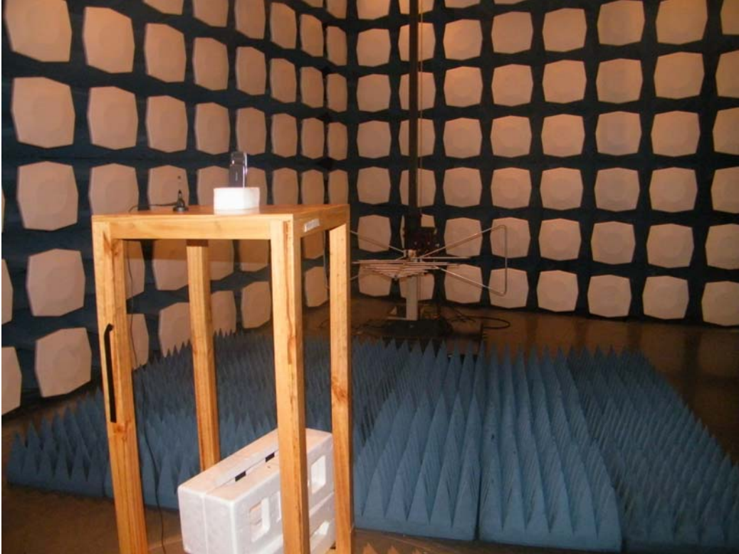
Picture 2: Radiated Spurious Emissions Test setup
